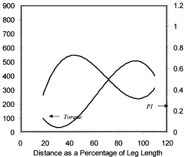
FIGURE 2. Torque (N-m, shown in the left vertical axis), and performance index (right vertical axis) plotted against distance (bottom axis) as a percentage of leg length.
