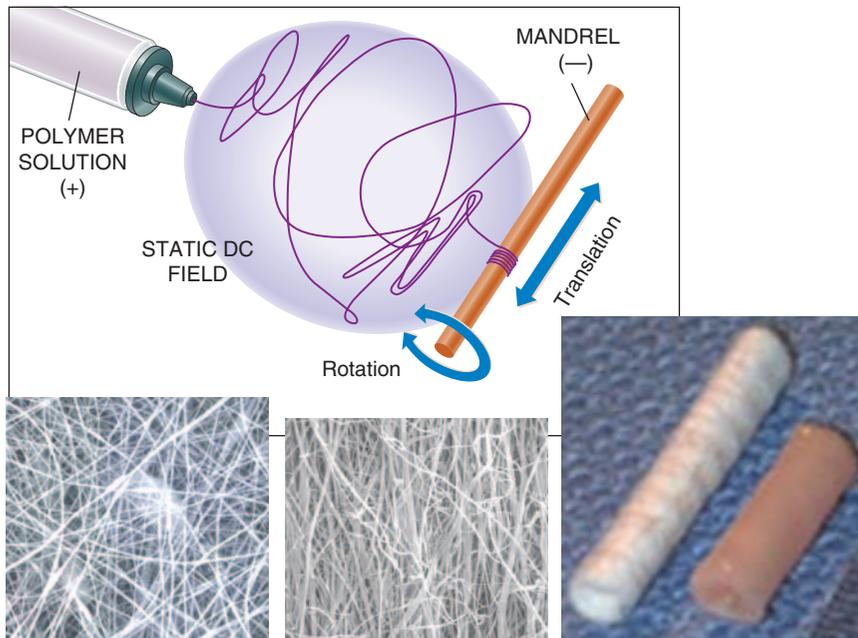
In **electrospinning**, a key component is the collection mandrel. Manipulating the rotational speed and translation of the mandrel allows the fabrication of random (*left*) or aligned (*middle*) collagen nanofiber scaffolds for use in applications such
